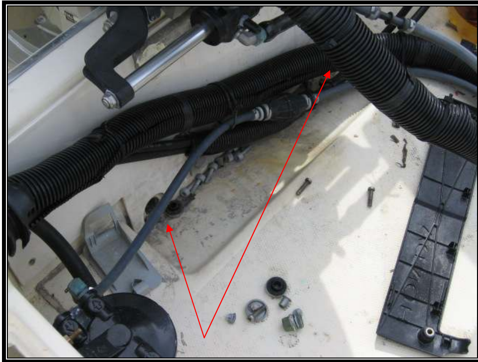
Scupper drains are port and starboard in well; The top of the well is 1/2" above top of scupper;
