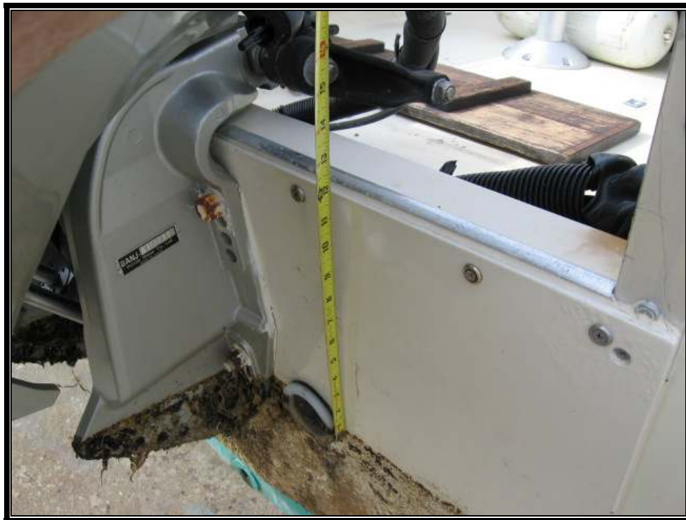
Freeboard aft = 12" +/- Note waterline near top of scupper
