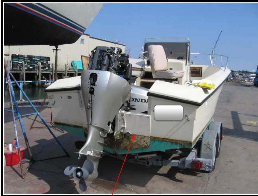
Note location of waterline/scupper drain – This allows water to enter the vessel when it is afloat
