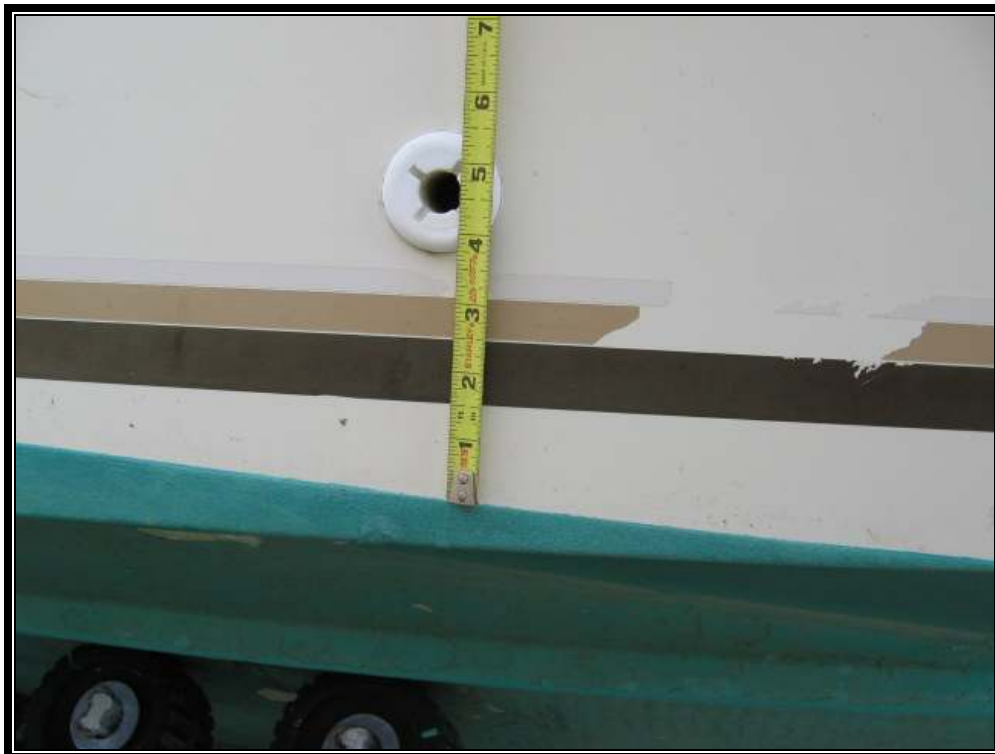
Scupper drains are port and starboard in well; The top of the well is 1/2" above top of scupper;
