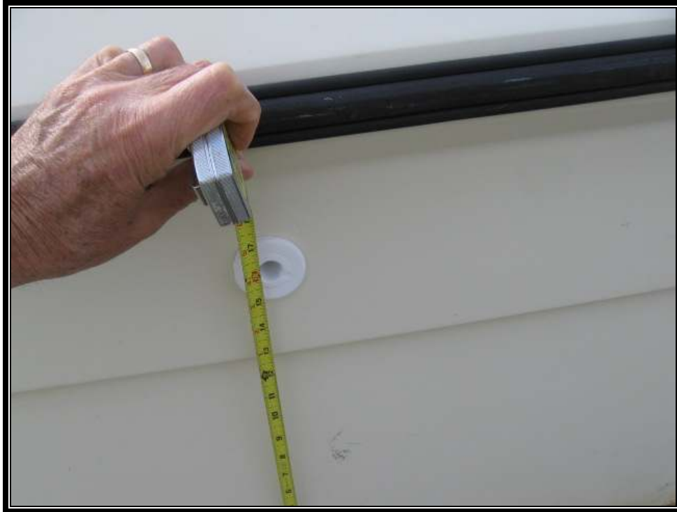
Bilge pump discharge fitting (16" +/- above waterline)
