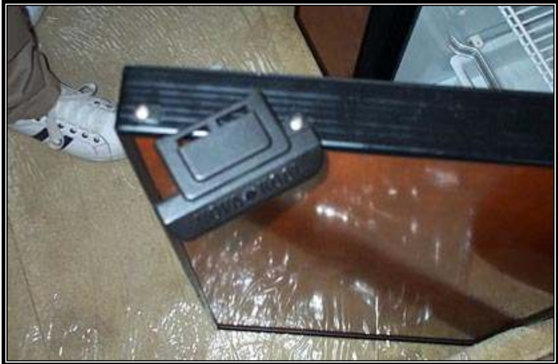
Broken Refrigerator Handle
