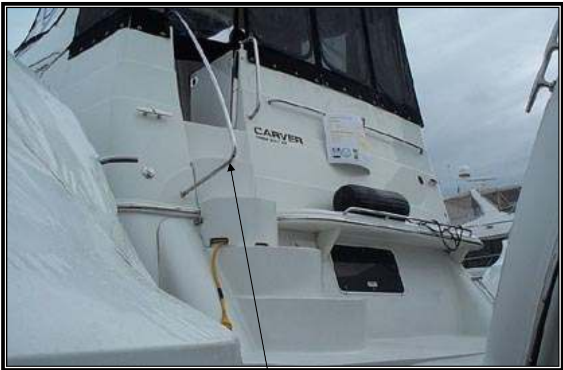
Loose Hand Rail
