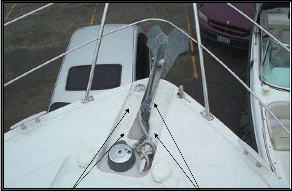
Small Areas of Elevated Moisture Meter Readings
