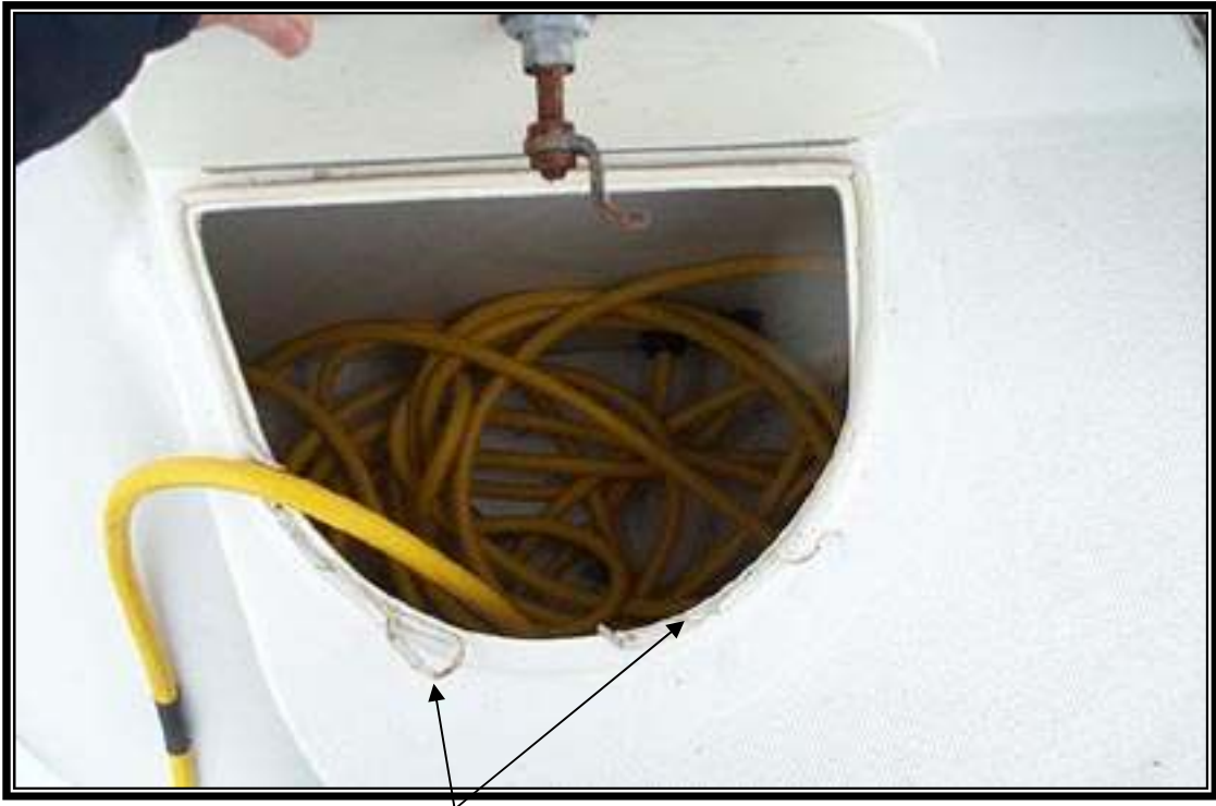
Deteriorated Cover Seal at Power Cord Storage Locker
